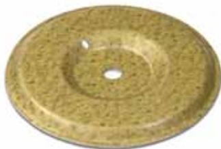
*In a short 2-step process, UltraPly TPO InvisiWeld plates are used to attach the Firestone insulation or cover board to the roof deck. Then the TPO-coated plates are welded to the underside of the UltraPly TPO membrane through patented heat induction technology.*
