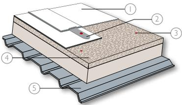
1. Firestone UltraPly Platinum TPO with Wide-Weld™ Seam Technology
