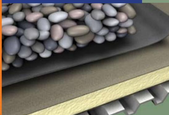
**Ballasted** systems are perfect for installations where speed and economy are prime considerations, and the substrate is capable of supporting the system's dead load. Slope must not exceed 2" (50.8 mm). Insulation and membrane are loose-laid with the membrane fastened only at the perimeter. Recommended ballast is smooth, water-worn rocks.
