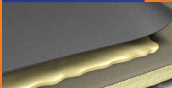
**Fully adhered** systems are ideal for roofs with unusual or odd-shaped contours, where mechanical penetration of the membrane is not desirable, yet exceptional wind performance is needed. Once positioned over the substrate, the back of the membrane and the substrate are coated with GenFlex bonding adhesive, allowed to dry, carefully rolled back into position and broomed into place.
