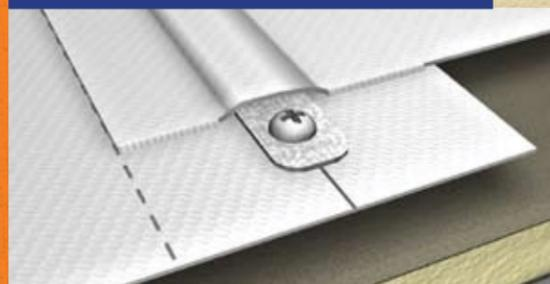
**Dual-Weld** offers even higher wind-uplift performance than single-weld seams, which create unequal, or asymmetrical, loading in the attachment area. GenFlex's patented Dual-Weld technology balances the wind load throughout the seam area, eliminating the stress around the fasteners and along the seams. By directly transferring the load to the in-seam fastening system, performance and uplift ratings improve.
