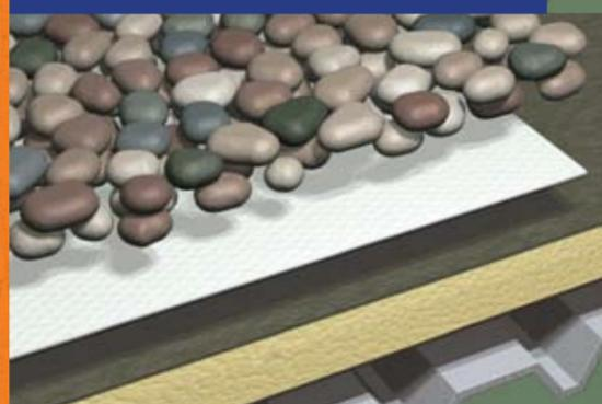
**Ballasted** installation is perfect when a job needs to be done fast and inexpensively. Insulation and membrane are loose-laid with the membrane fastened only at the perimeter. Recommended ballast is smooth, water-worn rocks. Substrate must be capable of supporting the dead load of the system.
